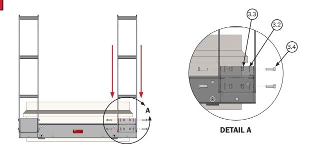
**STEP 3.** Determining the Support Tube Configuration. (See Illustration A and Illustration B)
